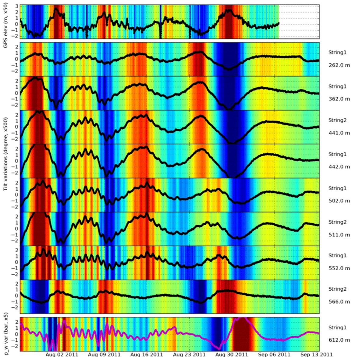
**Figure 1.** Borehole observations from drill site FOXX on the Greenland ice sheet. Shown are vertical surface displacement (top stripe), sensor tilt variations (extra motion superimposed on long-term trend), and basal water pressure (bottom stripe). Background coloring highlights the variability of the plotted curves, ranging from blue (low values) to red (high values).
