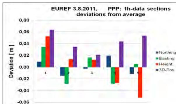
**Figure 2.** Comparison of 1-hour data sets of Static GPS solutions with PPP.
