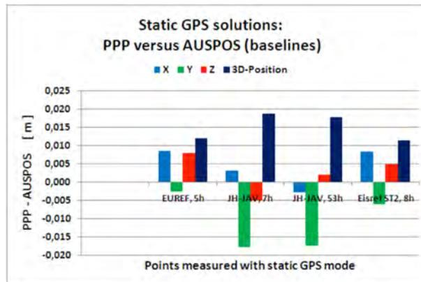
**Figure 1.** Comparison of Static GPS solutions between PPP and "true" values from AUSPOS baseline processing.
