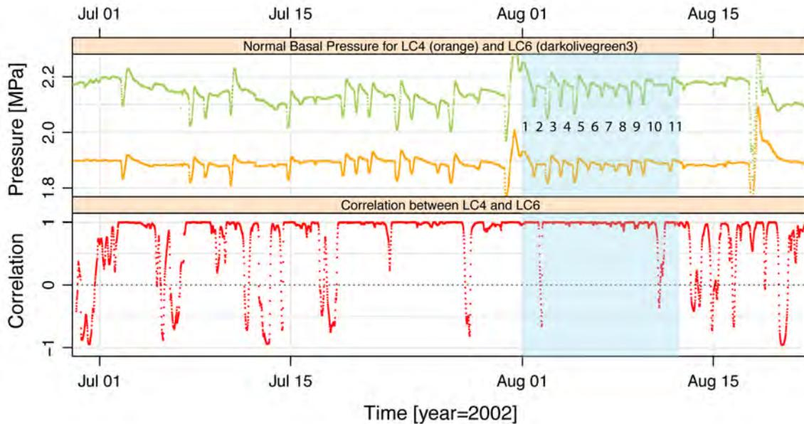
**Figure 2.** Time Series of Normal Basal Pressure from Load Cells LC4 (orange) and LC6 (green) and their correlation with a rolling window of 12 hours (plotted below). The part highlighted in blue indicates a strong diurnal signal with the observed number of cycles.
