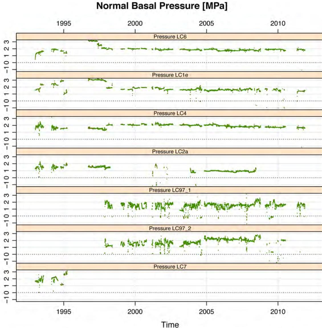
**Figure 1.** Time Series of Normal Basal Pressure is shown for the seven different load cells (left-hand side).
